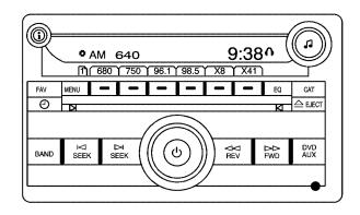
The DVD player is part of the radio and is located in the center of the instrument panel.
